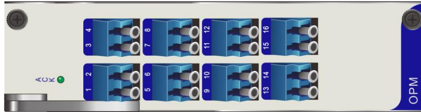
16 way OPM power meter board
